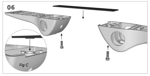
Place the steel strap onto the upper wrists, with the raised areas of the straps slotting into the holes on the upper wrist, *Fig C*. Fully tighten the M8x25mm bolts. (*Repeat with all upper wrists and steel straps*)
