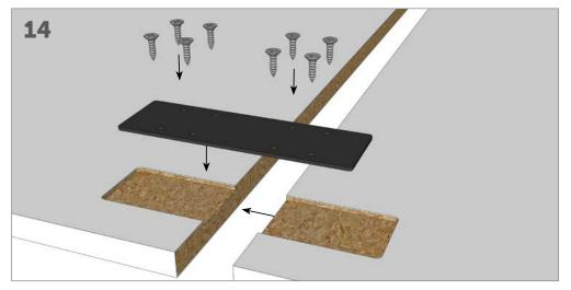
For multi piece work surfaces, use the table top bracket plates, and M5x20mm screws to join together as one solid piece. This should be done with the work surface sitting on the frame in its final position.
