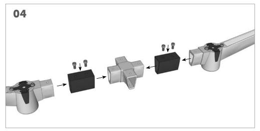
Using 2 T tubes, connect the assembled centre feet to the bottom cross connector, and fully tighten the 4 M8x16mm bolts.
